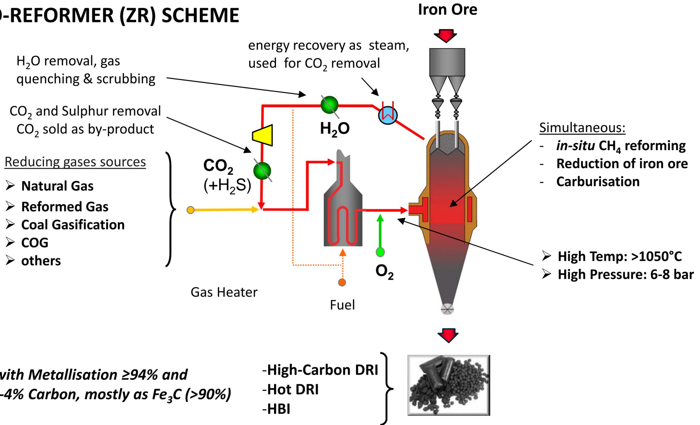
***DRI with Metallisation ≥94% and 1.5%-4% Carbon, mostly as Fe<sub>3</sub>C (>90%)***
